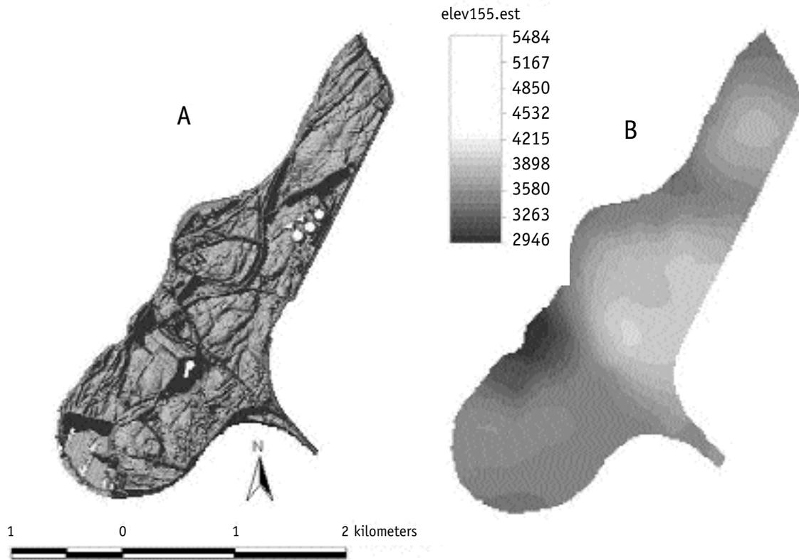
**Figure 3** A comparison of elevation data (mm above local reference) obtained from Laser altimetry of part of the Maas floodplain, (courtesy Dutch Meetkundige Dienst) and interpolation by kriging. Left: 5 x 5m resolution, right: surface interpolated from 155 surface measurements to a grid of 20 x 20m. Clearly, the high resolution surface (left) gives much more information over surface structures and ecological differences than the low resolution surface (right).
